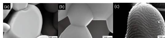
Fig. 1 Surface structures of porous FeCo prepared by LMD at (a) 600 °C, (b) 700 °C, and (c) 800 °C.
